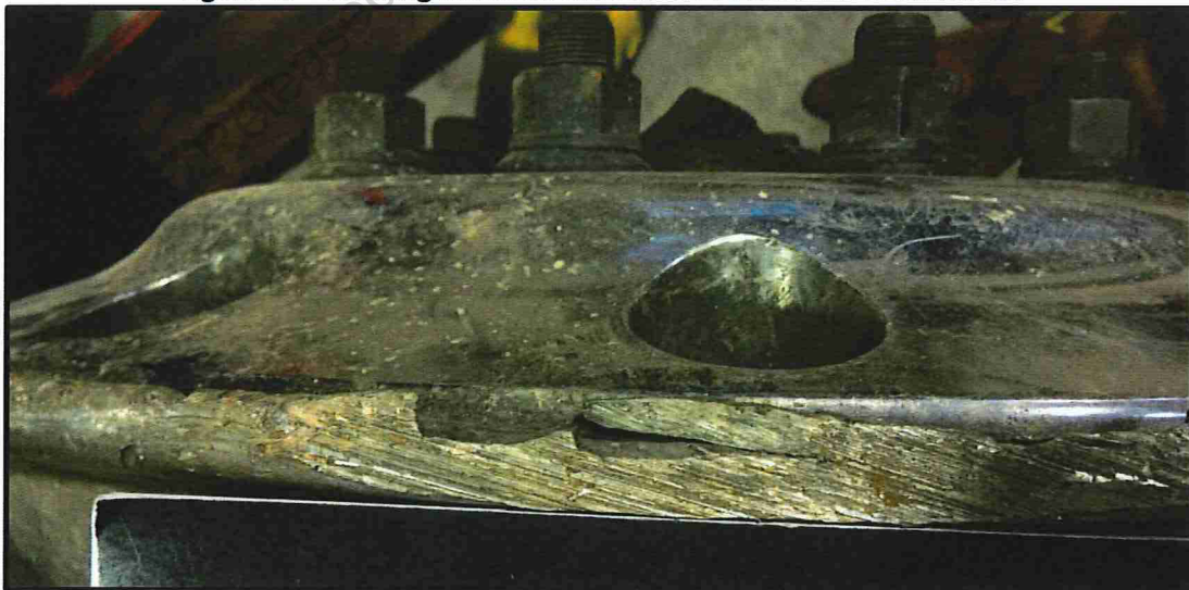
Figure 45 – Grinding marks on the rim of the left hand front wheel.
