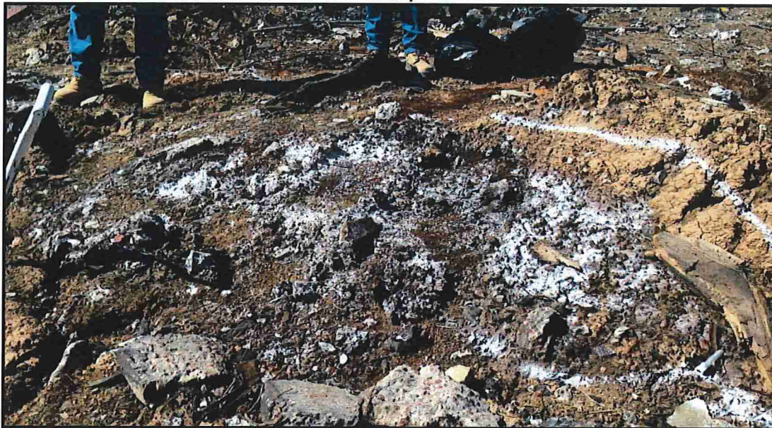
Figure 53 – Ammonium nitrate samples RB010, RB011 and RB012 under prime mover (white areas).
